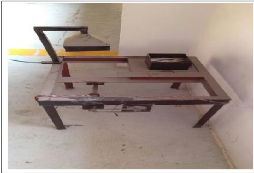
Fig.4. radiator tube cleaning machine
