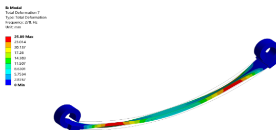
Figure 8 3 rd Mode Shape of Free Vibration of Composite Leaf Spring.
