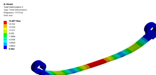
Figure 7 2 nd Mode Shape of Free Vibration of Composite Leaf Spring.
