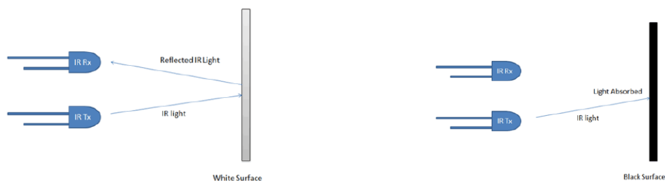
Fig.3:-IR Transmitter and IR receiver sensors working
