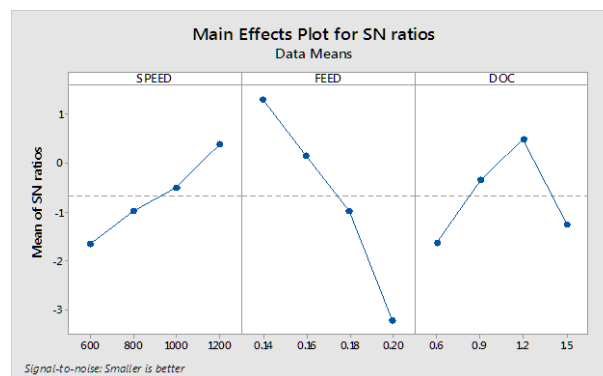
Fig 11 Response Main effects plot of SN ratios of Ra
