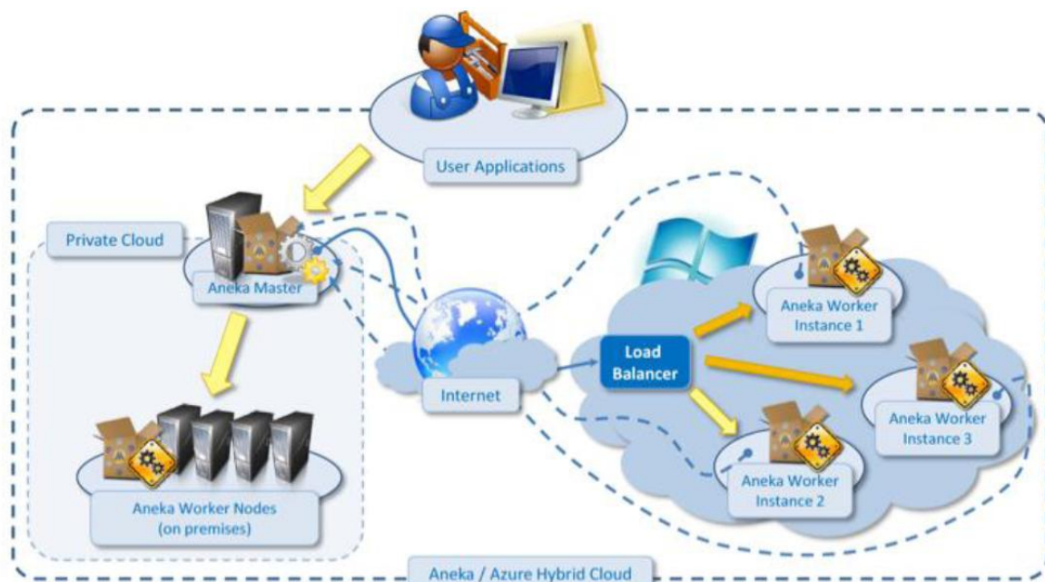
Figure 2: Schematic of Aneka/Azure Interaction for data analytics application
