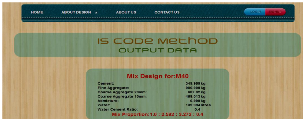
Fig.2 Image of an output jsp file for IS code mix design
