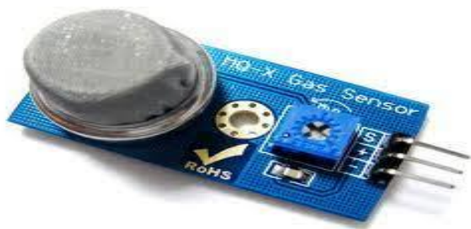
Figure 2.6: MQ-X Gas Sensor module detects gas leakage
