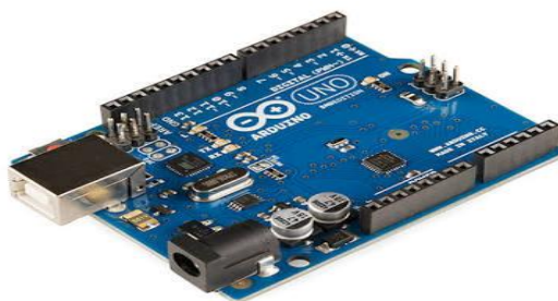
Figure 2.2: Arduino is an open-source electronics platform or board and the software used to program it.
