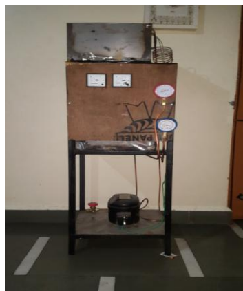
Fig.2. Experimental Setup of Heat Pump
