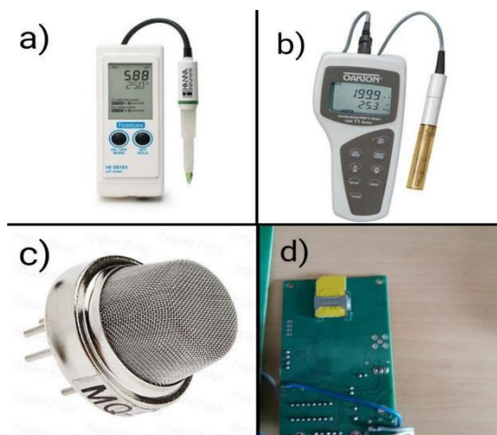
Figure 3. a) pH meter b) TDS meter c) Gas sensor
