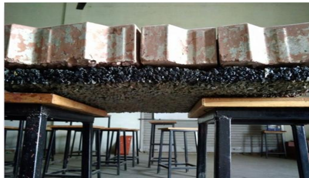
Fig. 6 Pervious Pavement with interlocking bricks
