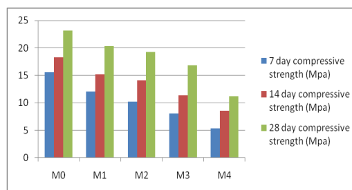
Graph 1: for compressive strength of concrete
