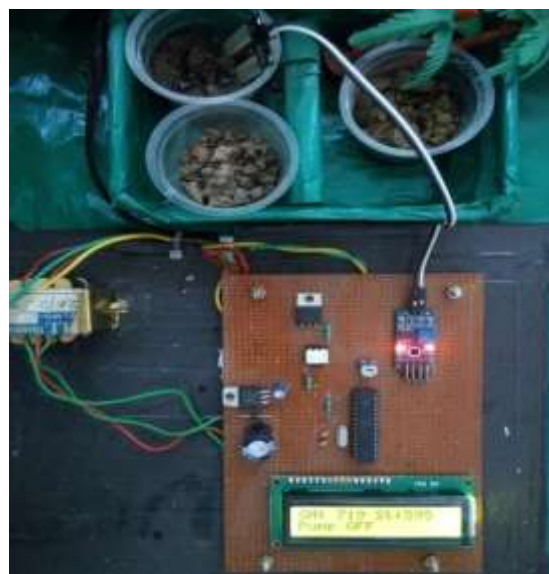
Fig.8 LCD indication when the soil pot 3 is wet
