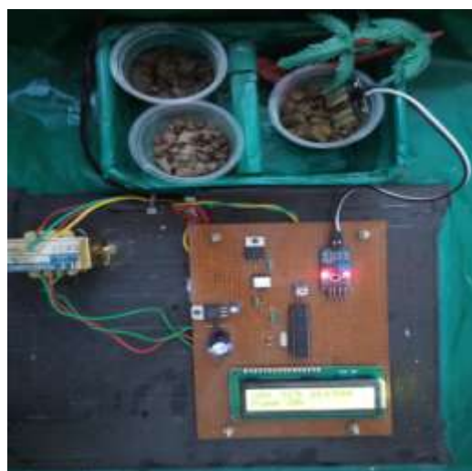
Fig.6 LCD indication when the soil pot is dry
