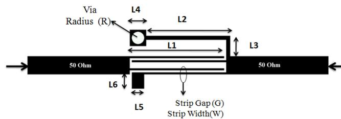
Fig. 1. Schematic of proposed filter. Substrate:  $\epsilon_r = 9.2$ ,  $t = 1$  mm.
