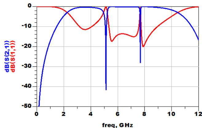
Fig.5  $S_{11}$  &  $S_{21}$  of Proposed Filter
