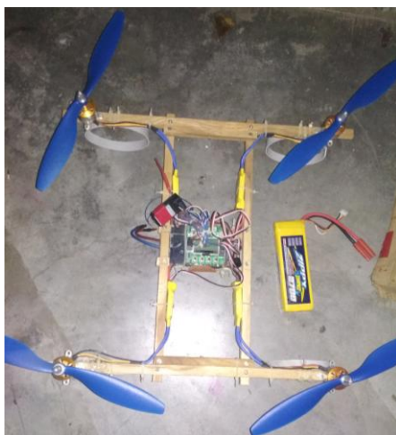
Fig.9 Quadcopter structure (rest view)
