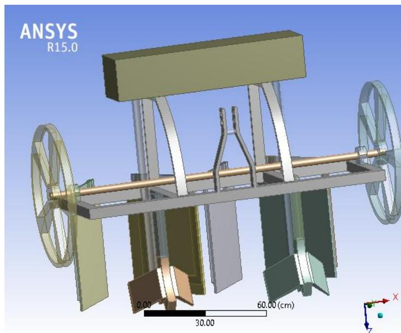
Figure 2. ANSYS design of sugarcane planter
