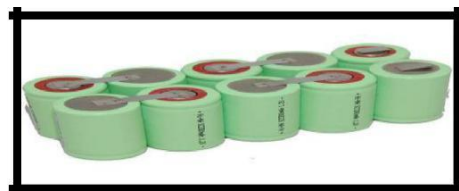
Fig-3: Inside of a 12V battery pack
