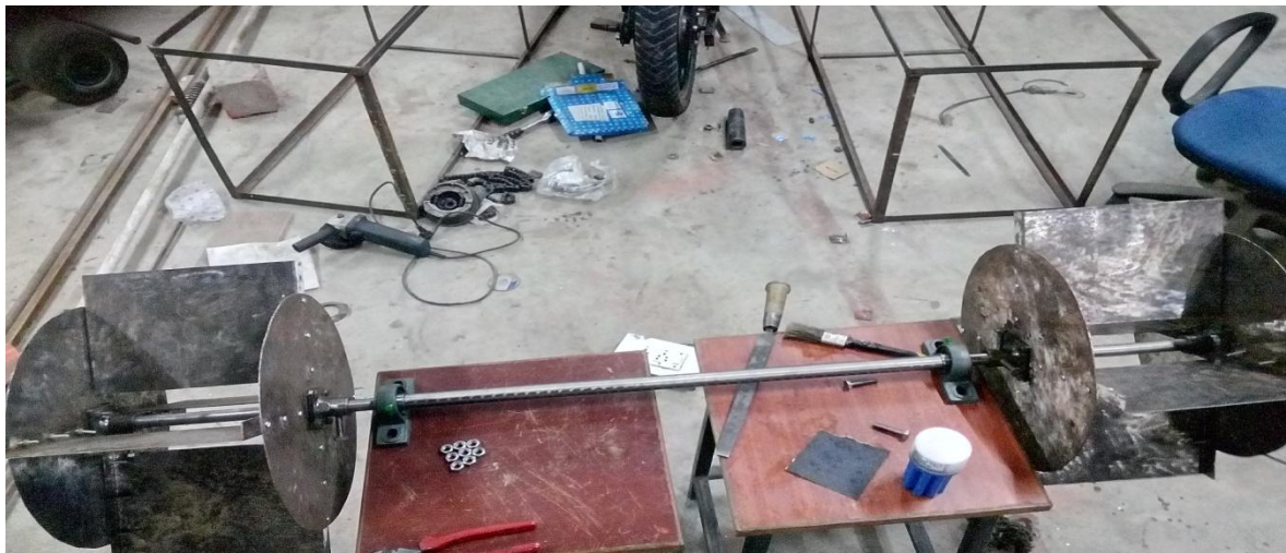
Fig 3: Blades aligned on a shaft and mounted by the end bearings
