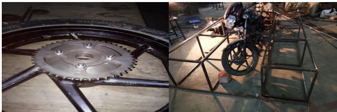
Fig 2: Sprocket adjusted at rear wheel for driving blades & front view of bike
