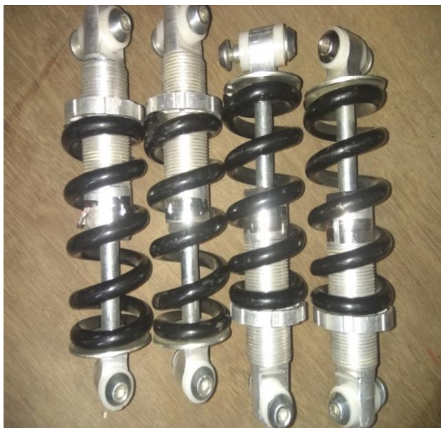
Figure 2: Coil suspension system
