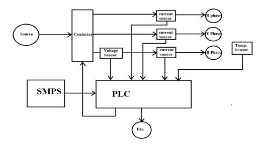
FIG (1) BLOCK DIAGRAM OF SELF HEALING PROTECTION SYSTEM OF INDUCTION MOTOR BY USING PLC
