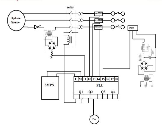
FIG (2) CIRCUIT DIAGRAM OF SELF HEALING PROTECTIONSYSTEM
