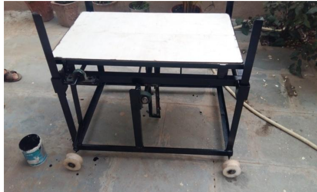
Fig.1 Actual Photograph of Flexible Trolley
