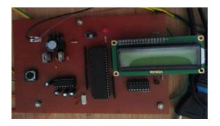
We use Copper clad PCB(Printed Circuit Board) to connect electronic component or electrical component are soldered on PCB by using conductive tracks and other features etched from one or more sheet layers of copper laminated onto and between sheet layers of a non-conductive substrate.
