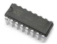
A motor driver is an integrated circuit chip which is usually use to control motors. Motor driver act as an interface between microcontroller and motors. The L293D motor driver is most commonly used and it designed to control 2 DC motors simultaneously. L293D has 16 pins.
