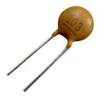
A ceramic capacitor is a fixed value capacitor in which ceramic material act as dielectric.
