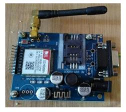
It is used to send message to the garbage depot if the Garbage Can exceeds the set threshold level. With the help of GSM module interfaced, we can send short text messages to the garbage van driver. GSM module is provided by sim uses the mobile service provider and send message to the respective authorities as per programmed. It operates at either the 900 MHz or 1800 MHz frequency band. We give supply 12v DC.
