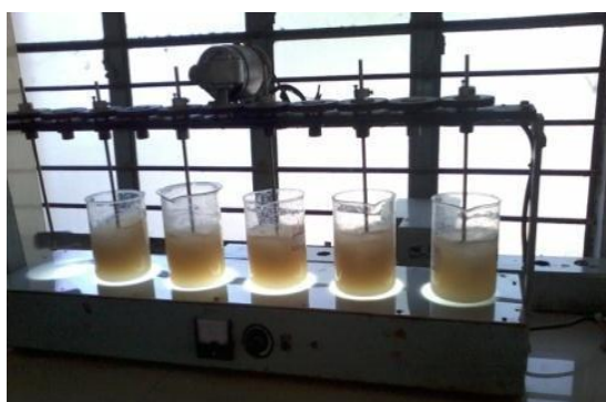
Fig.2 Schematic view of conventional jar test apparatus
