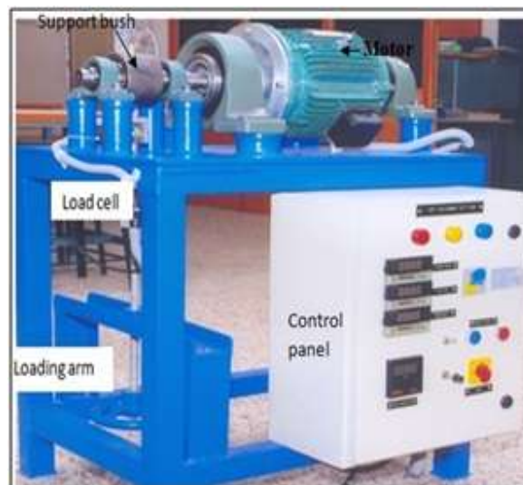
Figure 1(a). Dry bearing test rig
