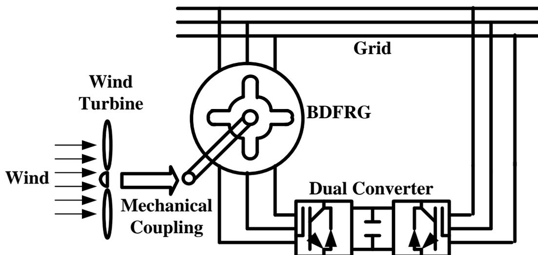
Fig. 1: Local grid connected BDFRG
