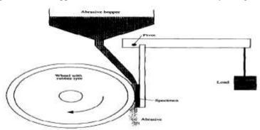
Fig 1.1. Schematic diagram of the rubber wheel abrasion testing (RWAT) apparatus described by ASTM G65 (Annual Book of ATSM Standards volume 03.02, pp. 247-259).
