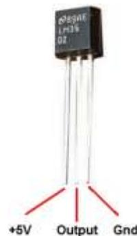
**Fig 3. Temperature Sensor**
