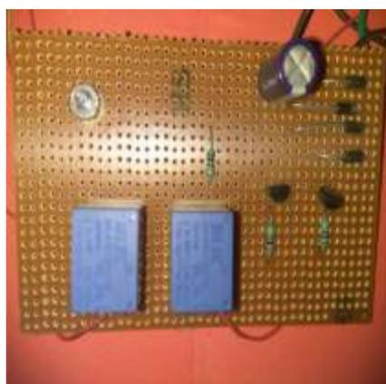
Fig 5. Relay Driver Circuit
