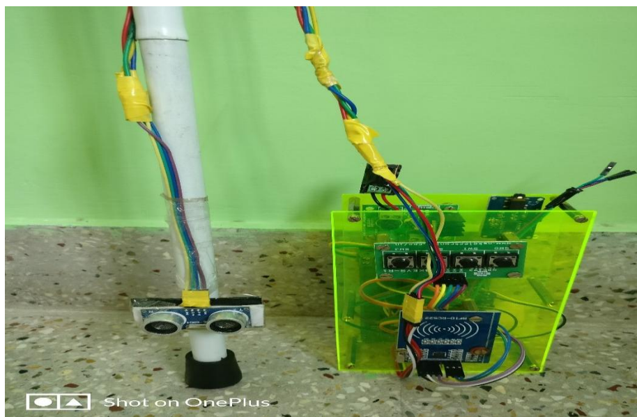
Working smart cane with gadget box for obstacle detection and product scanning
