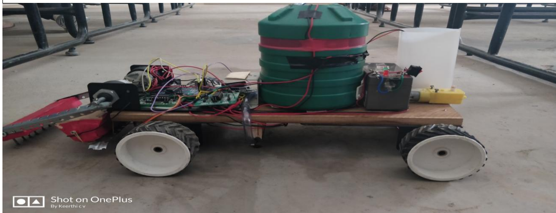
Fig:3.1.6 Multipurpose Agricultural Robot
