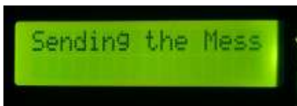
Fig.7: It will send the OTP message to Customer number through GSM module
