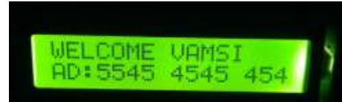
Fig.6: when fingerprint is matched with the database it will display customer details
