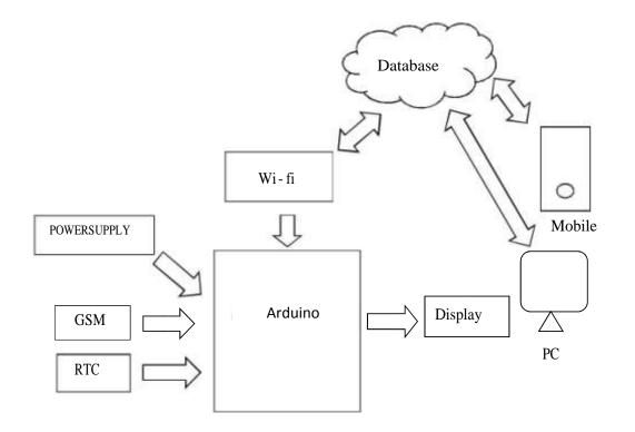
Fig.1: Proposed Block Diagram of implementation of Smart Display
