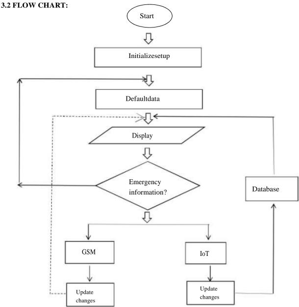
Fig 2: Flow chart of Smart Display system working.
