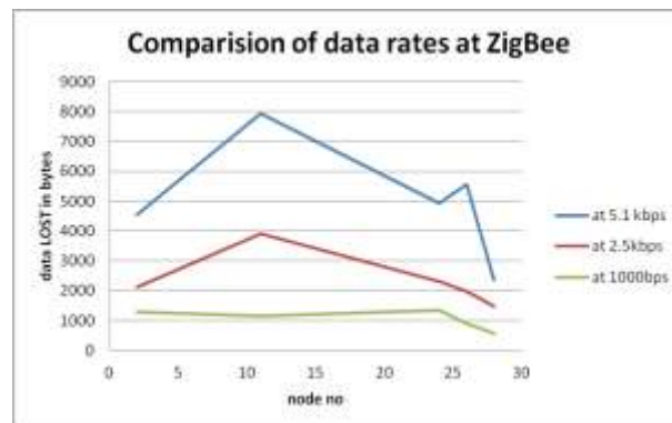
Fig.6: Data rates varying at ZigBee communication
