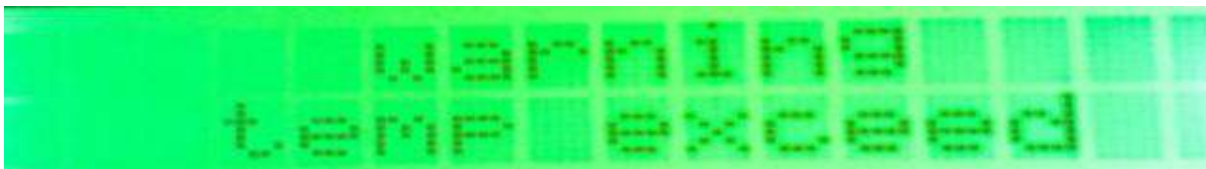
Fig.6: Warning after Temperature exceed
