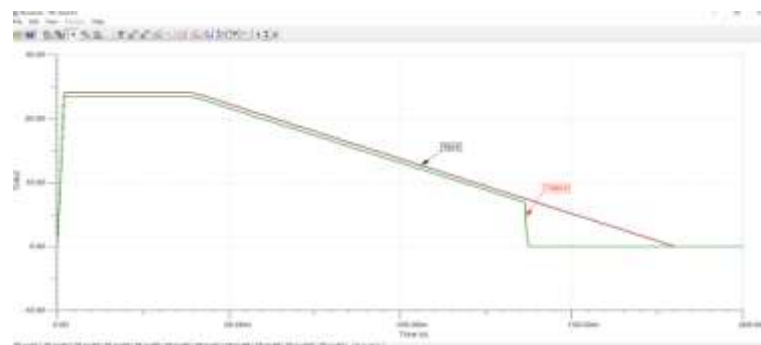
Fig 20: Simulation result for under voltage shutdown
