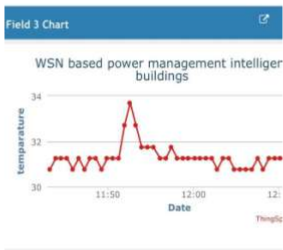
Fig.3: it has two fields date(time) and temperature. If the temperature is above a threshold value, the fan is switched on.
