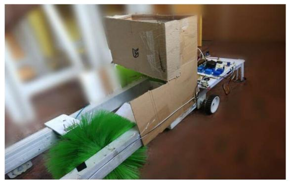
This robot cleans and collects the waste accumulated between the tracks, detects the crack in the track, detects obstacle present in front of the robot, sprinkles the mixture of water and disinfectant continuously after cleaning, gives red signal indicating that the robot is in cleaning process and gives green signal when cleaning is completed.
