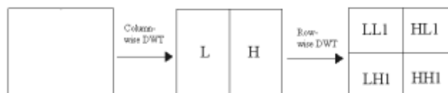
Fig.1: First level 2D-DWT generating four different outputs.
