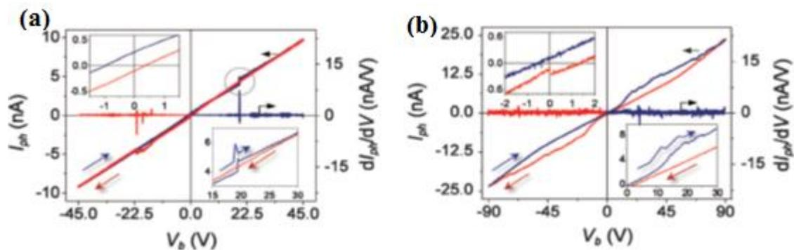
**Figure 3:** (a) I-V characteristics under global illumination on single-domain (b) and multidomain BFO (adopted with permission from ref. 15).
