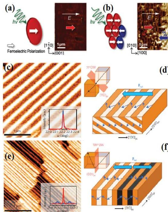
**Figure 1:**(a) shows in-plane PFM images of (110) BFO single domain and(b) (100) BFO multi-domains, net polarization directions are indicated by red and blue arrows (c, d) PFM image and x-ray curves of  $71^\circ$  domain walls (e, f) PFM and x-ray curves of the  $109^\circ$  domain wall arrays (adopted with permission from ref. 12,15).
