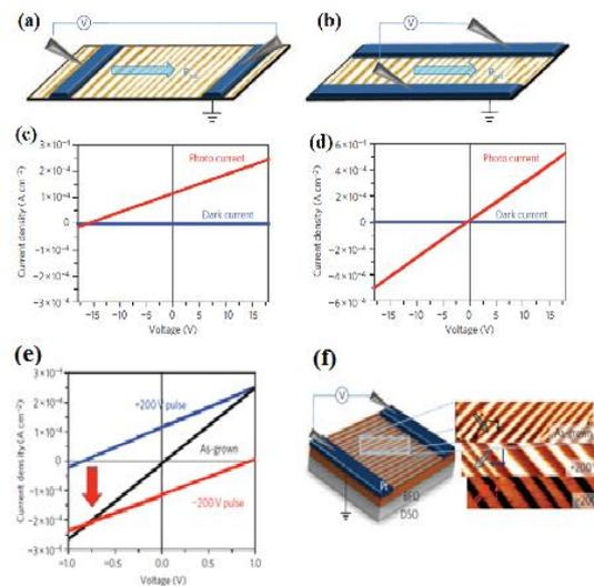
**Figure 2:** Schematics of the (a) perpendicular ( $DW \perp$ ) (b) the parallel ( $DW \parallel$ ) device geometries, (c) I-V measurements of the ( $DW \perp$ ) (d) and ( $DW \parallel$ ) devices, (e) domain-wall switching effect (f) corresponding PFM images of the as-grown (top panel), 200 V poled (middle panel), and 200 V poled (bottom panel) device structures (adopted with permission from ref. 12, 15).
