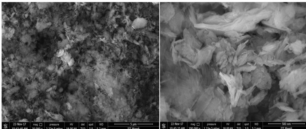
Fig. 3(a) SEM images for pure CuO nanoparticles
