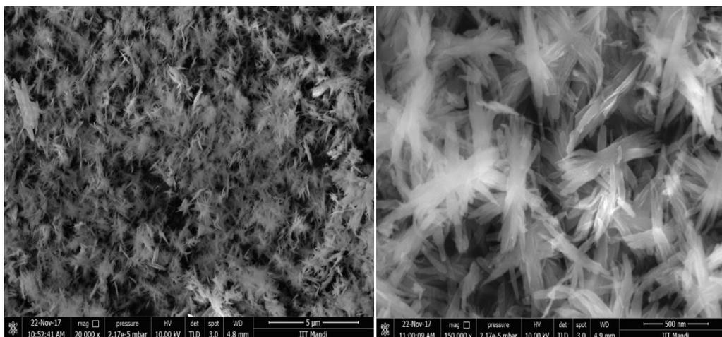
Fig. 3(b) SEM images for Zn-doped CuO nanoparticles
