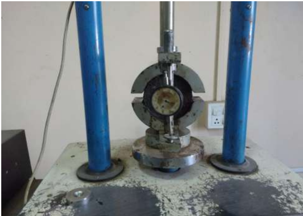
Figure 3.1 Marshall Stability test set up
