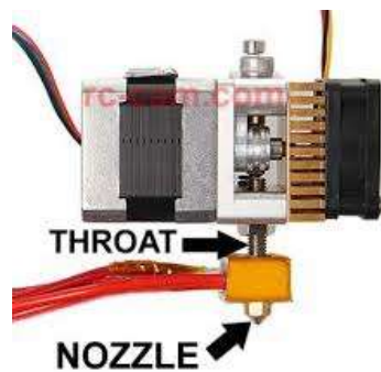
Fig. 4 Hardware Structure of MK8 Extruder
