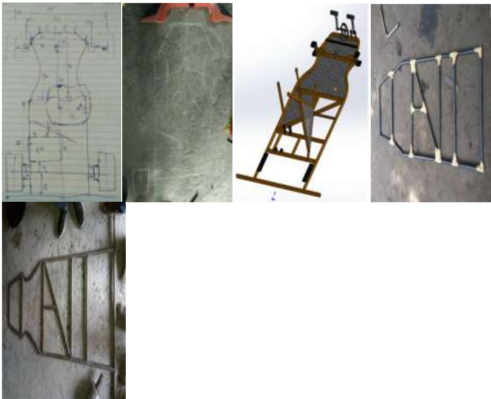
Fig1- Hand sketch Fig2- Floor plan Fig3- Final design Fig4- PVC Prototype Fig5;Developed chassis
