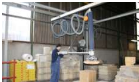
Fig 1.- Image showing lifting of solar panel using pneumatic gripper
