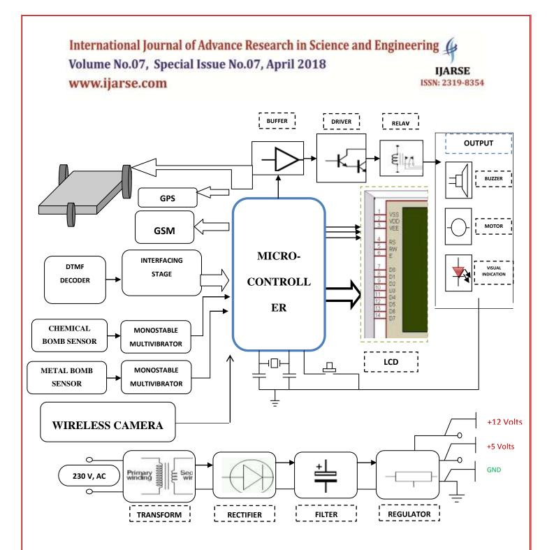
Fig 1.Block Diagram of Land Rover Robot.
