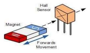
Fig 6.Head on detection.
