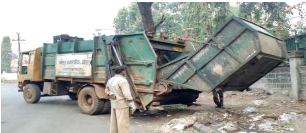
Fig. No.3- R.C. Truck lifting the Collection Bin in E-3 Ward, Kolhapur City
