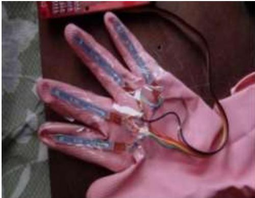
**Fig.9. Flex sensor Mounted on Gloves**
