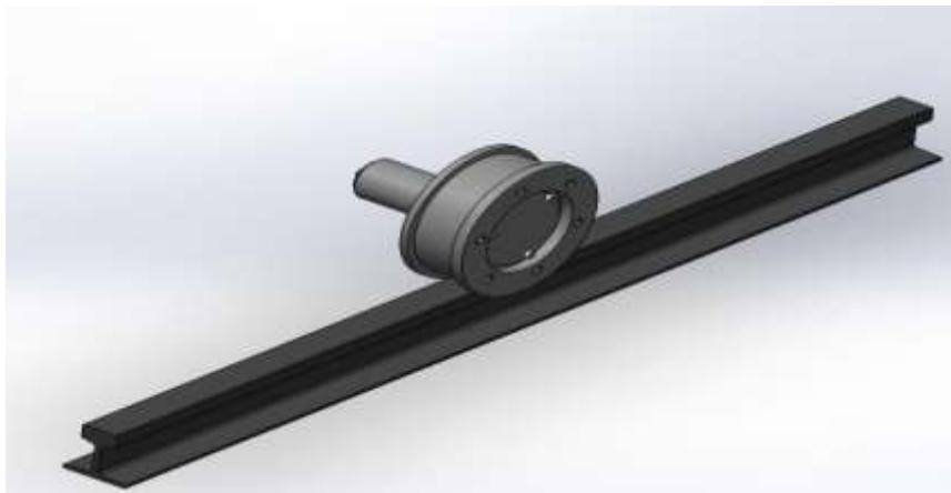
**Fig 3: Model of wheel for Rail transfer trolley**
