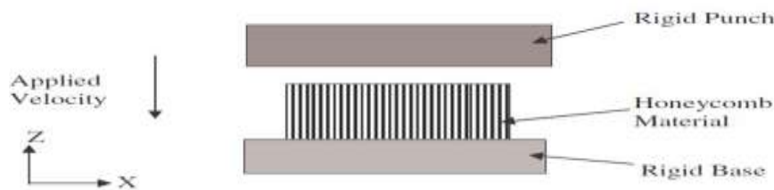
Figure 5: schematic diagram of honeycomb crushed in out-of-plane direction
