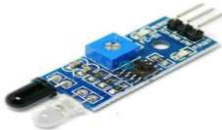
Fig.2.3 INFRARED SENSOR
