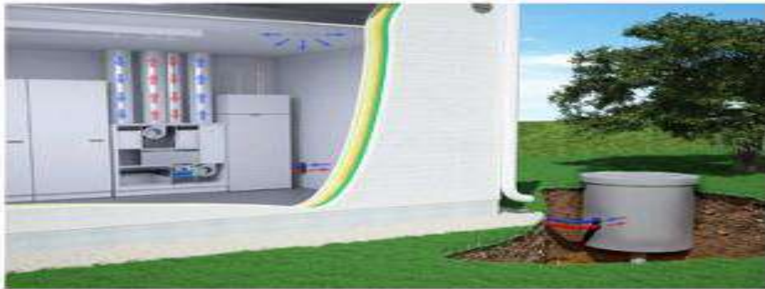
Fig. 7. Schematic diagram of ventilation systems with geothermal heat pump.
