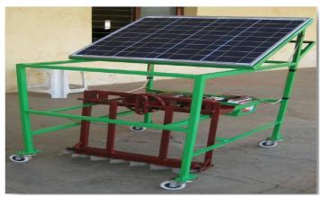
Sujendran .S, Vanitha .P developed automated machine for trimming the grass. The machine is use up of linear blade. The battery can be charge by using power supply and solar panel. IR sensor is used for detecting obstacle. In future the automation of the device will play a vital role in world wide.
